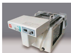
① Shaking Unit, BN300 ② Constant temp. water bath, BK400
